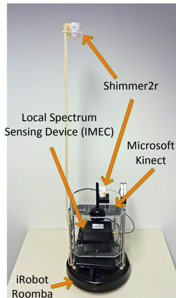
**Fig. 1.** TWISTbot with two BAN nodes
