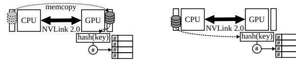
(a) Data and hash table in GPU memory. (b) Data in CPU memory and hash table in GPU memory.
