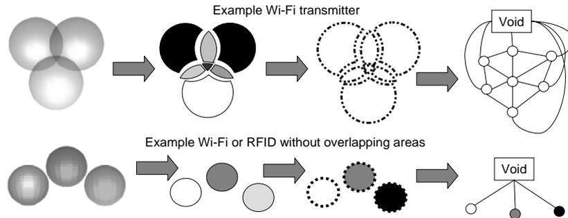
**Fig. 4.4.** Example for partitioning into cells and their representation in dual space For sensor systems covering the whole interior building area, the state “void” only represents the outside building environment. Fig. 4.4 illustrates the modeling of sensor space in the case of overlapping transmitter/sensor ranges.
