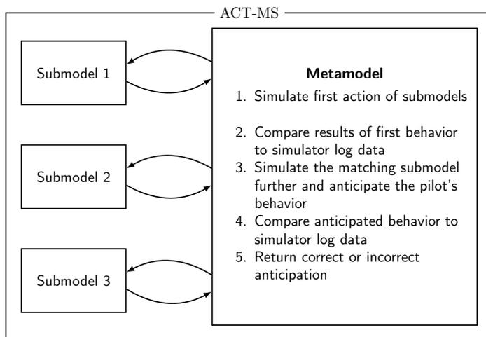
FIGURE 3: Concept of a metamodel and three submodels. The basic steps of a mental simulation and anticipation are denoted within the metamodel.
