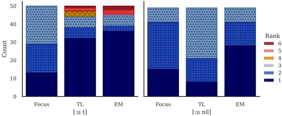
FIGURE 8: Results of the submodel selection in the ISM, denoted by the rank of how many submodels had to be simulated to match a pilot monitoring's action (TL = Thrust Lever, EM = Engine Master).
