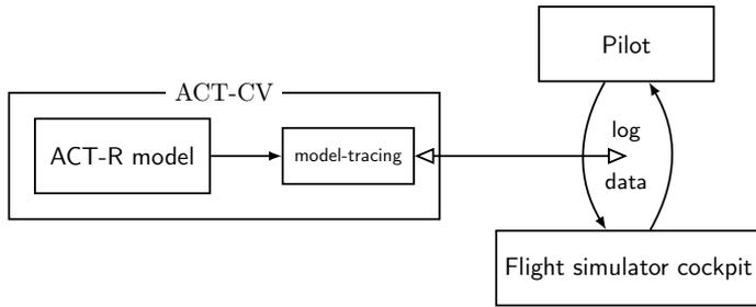
FIGURE 2: The cognitive model interacts during runtime with simulator log data containing simulator states and pilot actions in a process known as model-tracing.
