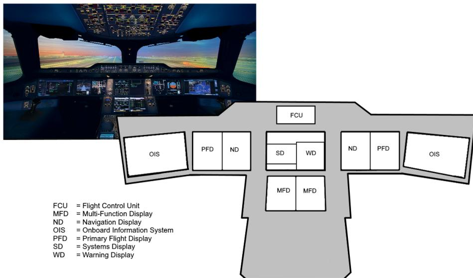
FIGURE 1: Display names for visual focus areas of the Airbus A350 cockpit layout used in the simulator study (copyright: Airbus).
